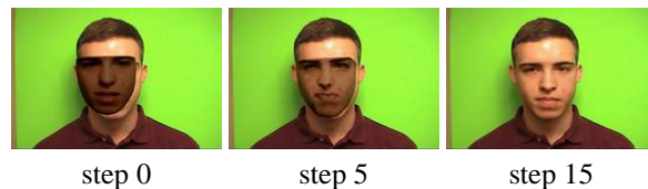
Fig. 3. Example of the AAM fitting algorithm. As the face mask better localizes the speaker's face, the reconstruction error decreases.
