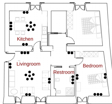
Fig. 1. The floorplan of the apartment for which the DIRHA prototype is being developed. The black dots represent the 40 microphones installed, namely 28 microphones on the walls and two pentagon-shaped arrays on the kitchen and livingroom ceilings.
