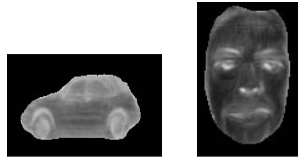
Figure 4. The variance of the reconstruction error for a morphable model for cars and faces is larger at areas of high complexity, like wheels and eyes, respectively.
