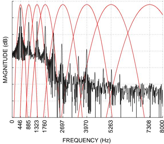
**Fig. 1:** Gabor filterbank with the estimated center frequencies  $f_c$  after the application of the iterative-ESA superimposed over Bb Clarinet spectrum for a 30 ms frame of the note A4,  $F_s = 44.1$  Hz.
