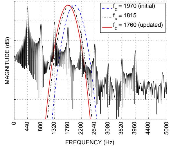
**Fig. 2:** Gabor filters superimposed over Bb Clarinet spectrum for a 30 ms frame of the note A4. The iterative-ESA for the fifth Gabor filter started at  $f_c = 1970$  Hz and after two iterations converged to  $f_c = 1760$  Hz which is  $4f_0$  for the note A4, with a difference of 210 Hz.
