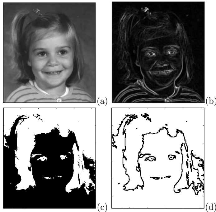
Figure 8: (a) Original image f with range in [0, 255] . (b) f \oplus B - f \ominus B , where B is a 3 \times 3 -pixel square. (c) Level set X = X_i(f) of f at level i = 100 . (d) X \oplus B \setminus X \ominus B . (In (c)-(d) black areas represent the sets, while white areas are the complements.)
