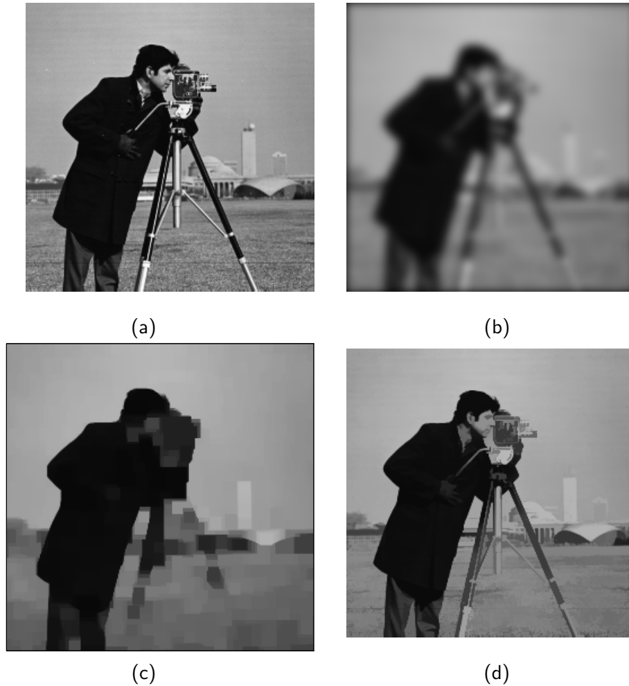
Figure 1: Linear and morphological image simplification. (a) Original image f ( 256 \times 256 pixels). (b) Linear convolution of f with a Gaussian. (c) Morphological clos-opening of f by a discrete disk-like structuring element. (d) Morphological reconstruction (of the leveling type) of f with respect to a marker which was the Gaussian convolution in (b). Both the linear and the morphological filterings were at the same scale. (The 'scale' parameter is defined as the variance of the Gaussian for the linear convolution, as the radius of the structuring element for the clos-opening and as the scale of the marker for the reconstruction filtering.)
